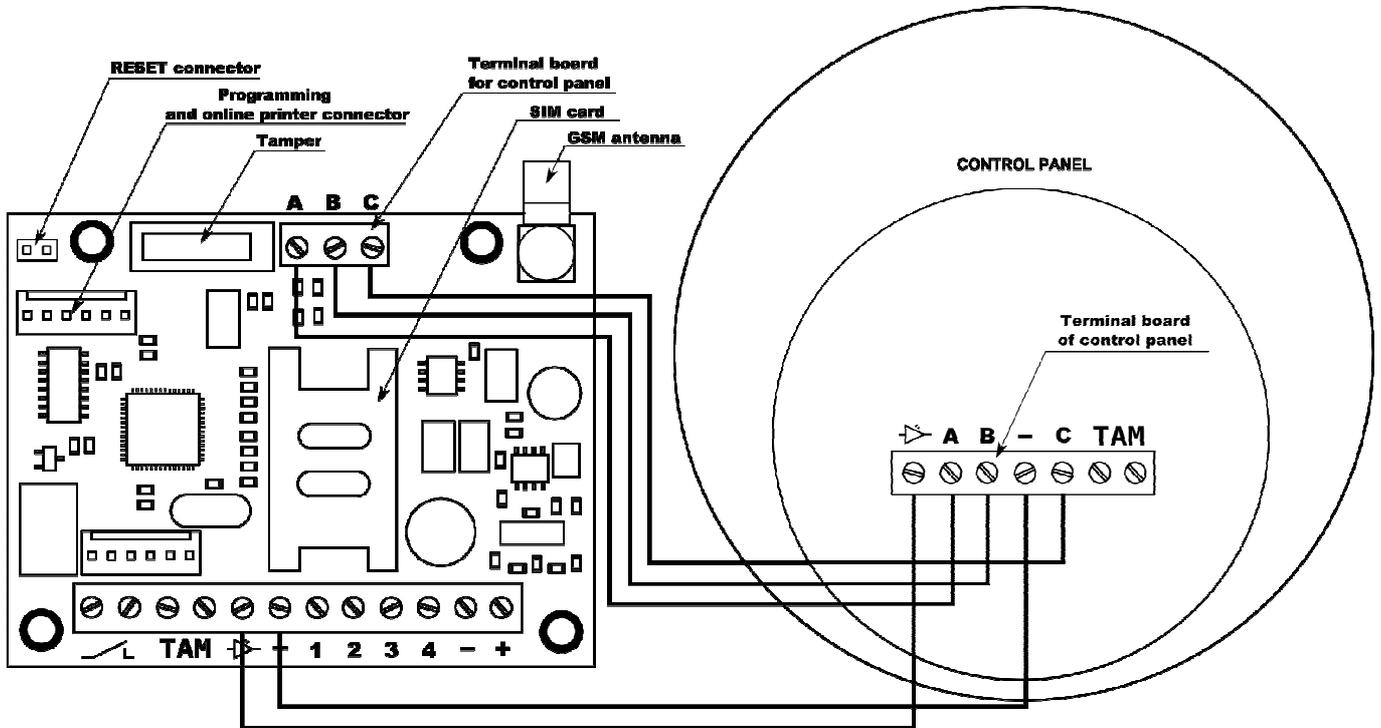
You will need to power the device from external backed up power source with nominal voltage of 12V or use the back-up power supply provided by manufacturer.
